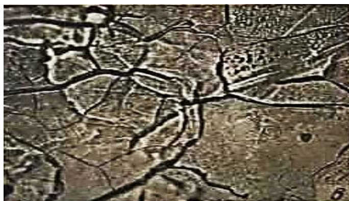
Figure 1.6. Deformation relief at 940 C temperature 500X
