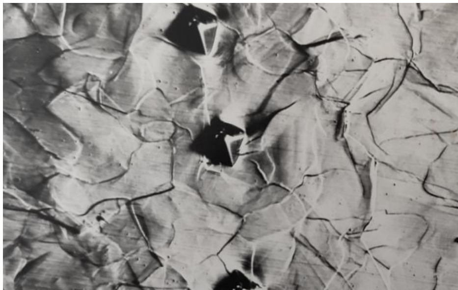
Figure 1.3. Deformation relief occurring at a temperature of 870 °C is 500 x
