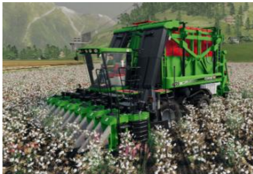
John Deere brand horizontal-spindle cotton harvesting machine (made in the USA) in cotton picking
