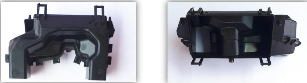
The physical property tests were conducted as follows: the part was subjected to 168 hours at  $95^{\circ}\text{C} \pm 3\text{K}$  and 24 hours at  $-30^{\circ}\text{C}$  in a temperature-controlled device. The results were positive.
