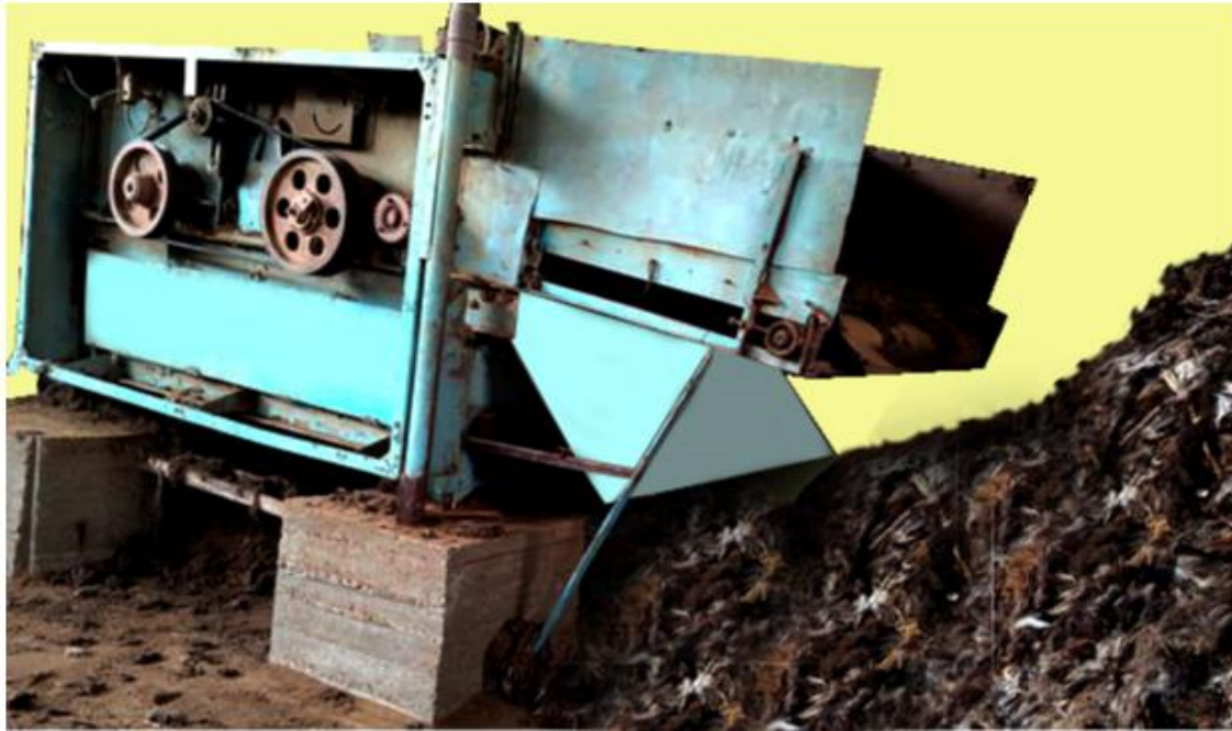
Figure 5. 2BT-150SH vibrating screen used at the Tinchlik enterprise.
