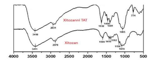
Figure 1. IR Spectra of Chitosan and Its Quaternary Ammonium Salt Derivative.
