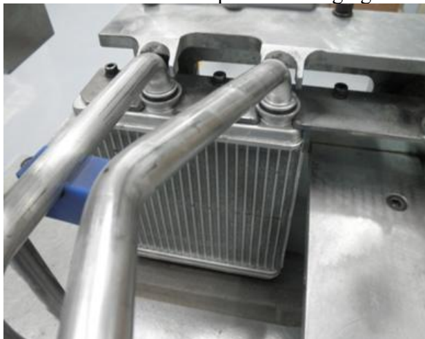
Fig1. Test machine car heating system
