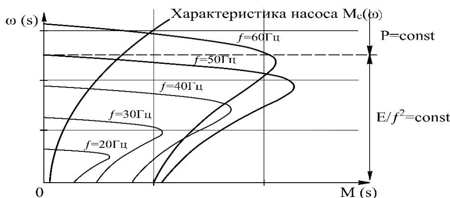
Figure 1. Mechanical characteristics of a frequency-controlled electric drive of a pump unit in the FC–AD scheme with an autonomous voltage inverter (AVI)
